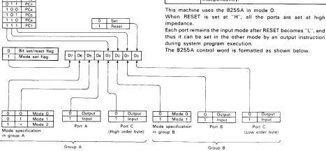
When using C port as an output port, any 1 bit only out of the 8 bits in the C port may be SET (H level)/RESET (L level) with the control word from the CPU.
